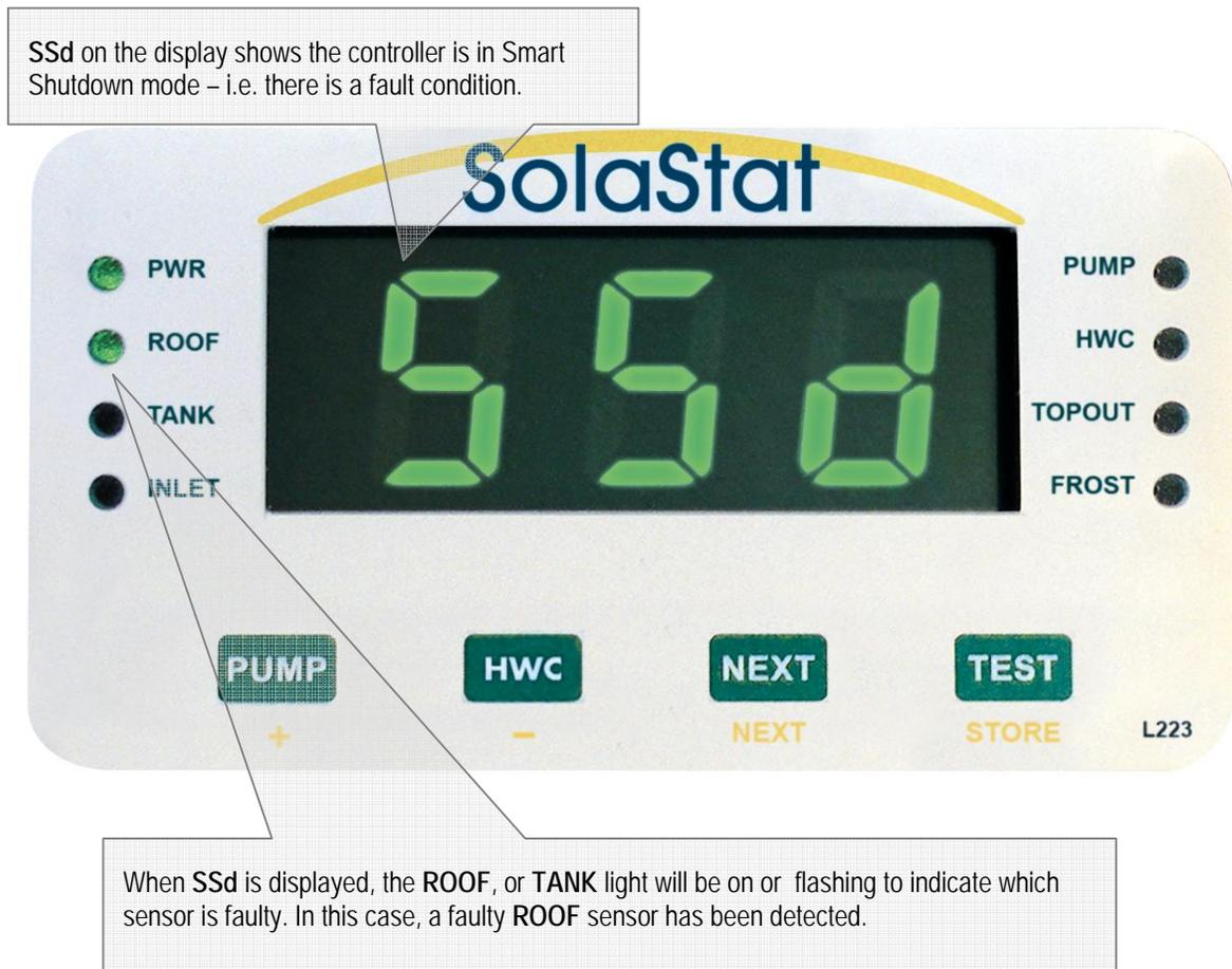
The Roof sensor temperature may reduce to a safe level by itself, and the unit will return to normal operation. SSd will no longer appear on the display.
