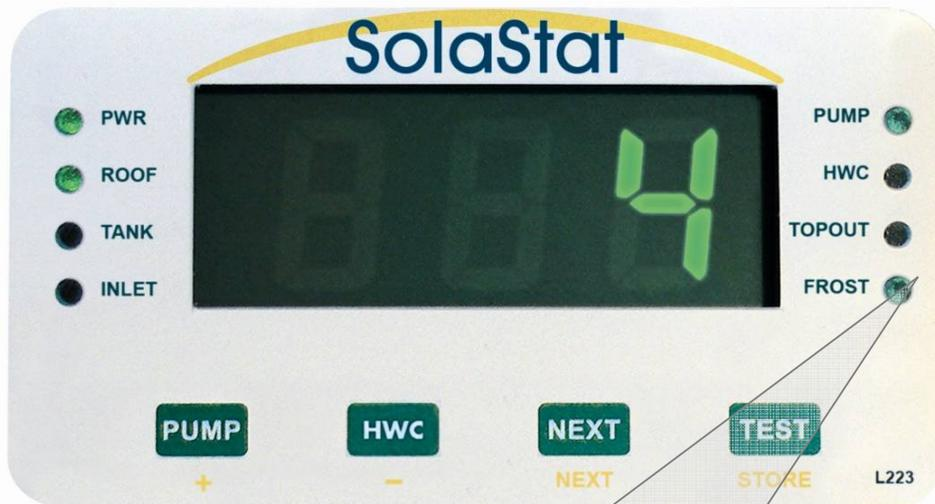
As soon as the collector reaches the **FROST** temperature, the **FROST** and **PUMP** lights will turn on.
