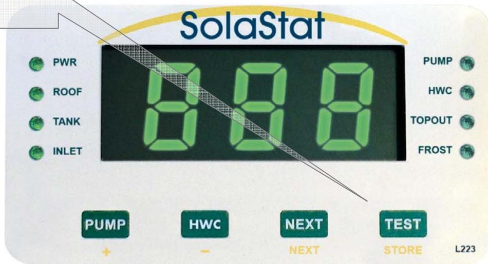
Then, all the lights will flash (except the **PWR** light), and the display will tell you how many times the pump has been activated (in this case, 123 times).
